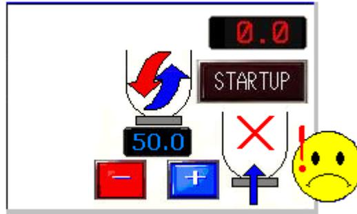
5. Turn the Inlet Blower OFF. The speed display will drop to 0, but it is only a forecasted speed. The actual speed may be checked at the drive itself (frequency output should be 0), or at the Drive States LEDs shown in Figure 2. If the "Running" status LED does not turn off until after the Inlet has finished ramping down to zero speed, the VFD must be re-programmed for "Coast to Stop".
