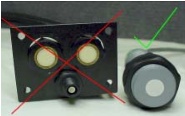
New sensor (right) is very easy to install
