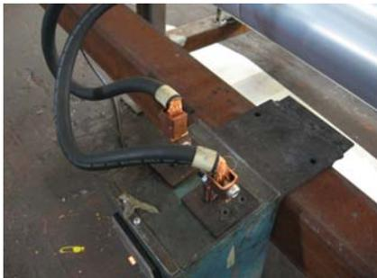
Exposed Slit-Seal Power Cables
